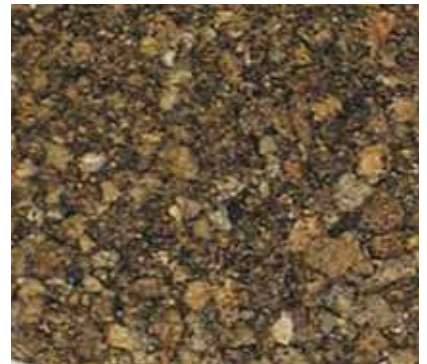
Plaisted Rooftop Garden Mixes are composed of a mixture of lightweight aggregate, compost and washed sand.
